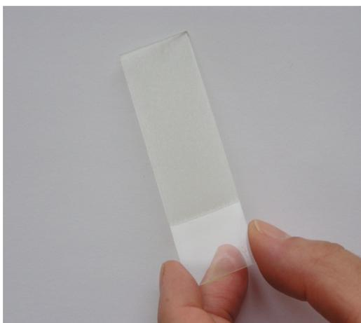
**Figure 1:** As-prepared gel titania thin film (1 layer) deposited on a soda-lime glass.
